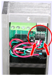
Jumper Setting for 12VDC Operation (Default Setting)
