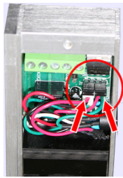
Jumper Setting for 12VDC Operation (Default Setting)
