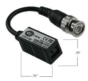
This passive pair balun with built in surge protector offers a convenient and cost effective solution to transmitting video signal over 2 wire conductor (we recommend CAT5E/CAT6 twisted pair). The COR-HTBE has a 4" pigtail which allows you to connect cameras to the DVR without space restraints. Boosts video signals up to 980ft (depending on cable quality and video signal) without power. Works with analog and analog high definition signals.
