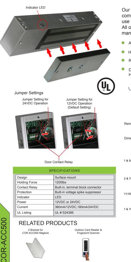
Our COR-ACC500 magnetic lock is widely used in commercial and industrial applications. It is perfect for use on doors and gates that close against a fixed stop. All of the lock components are carefully designed, manufactured, and tested to ensure superior quality.
